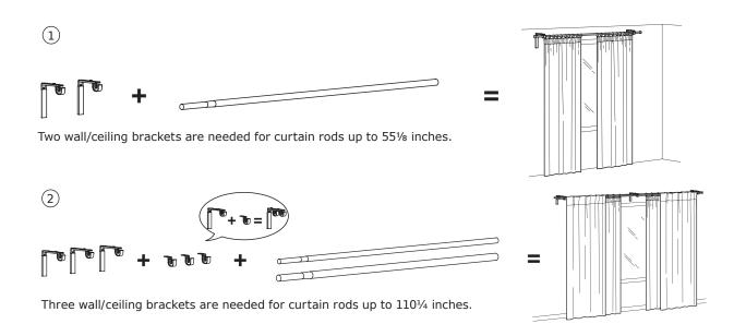
1. The brackets can be mounted on the wall or the ceiling. And the position of the curtain rod holder can be adjusted, allowing curtains to be hung either close to the window or farther out.
