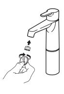
Before use: Unscrew the Aerator/Flow Guide with a coin and allow the water to run freely for a few minutes. Then screw the Aerator/Flow Guide back in place up to the stop DO NOT OVER TIGHTEN.
