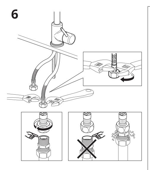
**English**IMPORTANT! Do not tighten too hard: this can damage hoses/pipes and washers.
