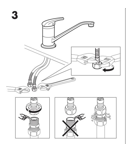
English IMPORTANT! Do not tighten too hard: this can damage hoses/pipes and washers.
