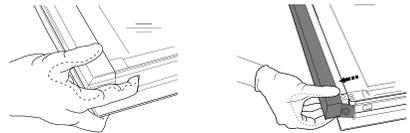
2. Lift and firmly hold the inner glass with both hands, remove it and place it on a soft surface before cleaning it. Do the same operation for the intermediate glass.
