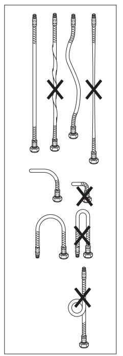
IMPORTANT! Do not tighten too hard: this can damage hoses/pipes and washers.
