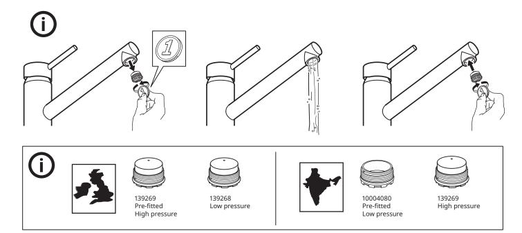
Before use: Unscrew the Aerator/Flow Guide with a coin and allow the water to run freely for a few minutes. Then screw the Aerator/Flow Guide back in place up to the stop DO NOT OVER TIGHTEN.
